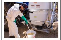
A suction probe is a great way to avoid having to lift a bucket to the top of a sprayer to tip chemicals into a tank. These require a bit of replumbing to make them work, but it's not too complex. We can help with that.
